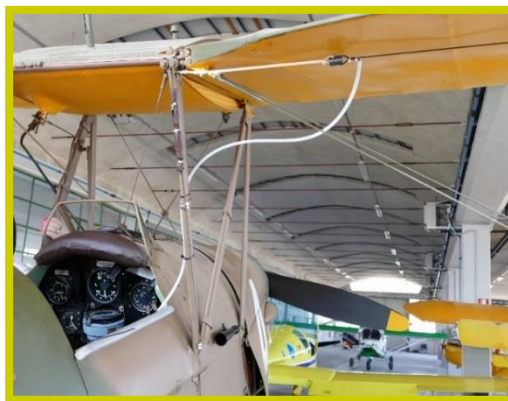
Photo N° 16 electrical insulator and insulating tube clamped on the interplane strut to allow the antenna cable to enter the observer's cockpit
