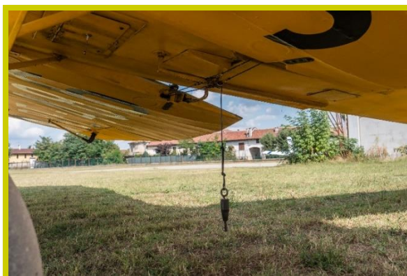
Photo N° 14 the 25-meter antenna, with a weight of about 300 g, which comes out of the biplane's cockpit
